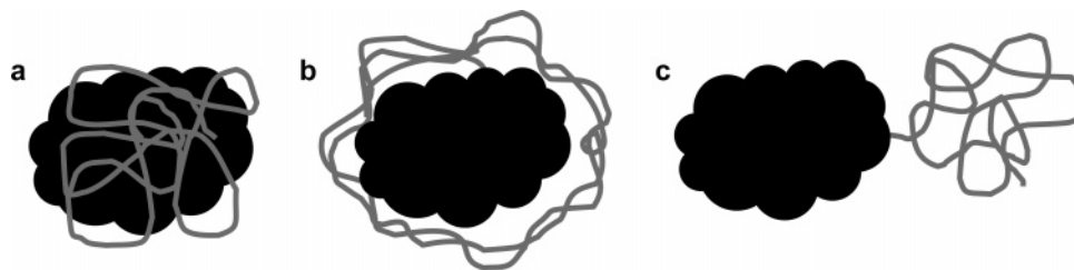
Figure 1. Three potential conformational states of linear–dendrimer diblocks in solution: (a) knitted coil, (b) encapsulated dendrimer, and (c) random coil.
